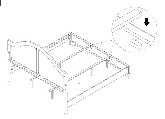
Adjust the leveling feet of the legs 5 to ensure all slats 4 are leveled and staying at the same level.
