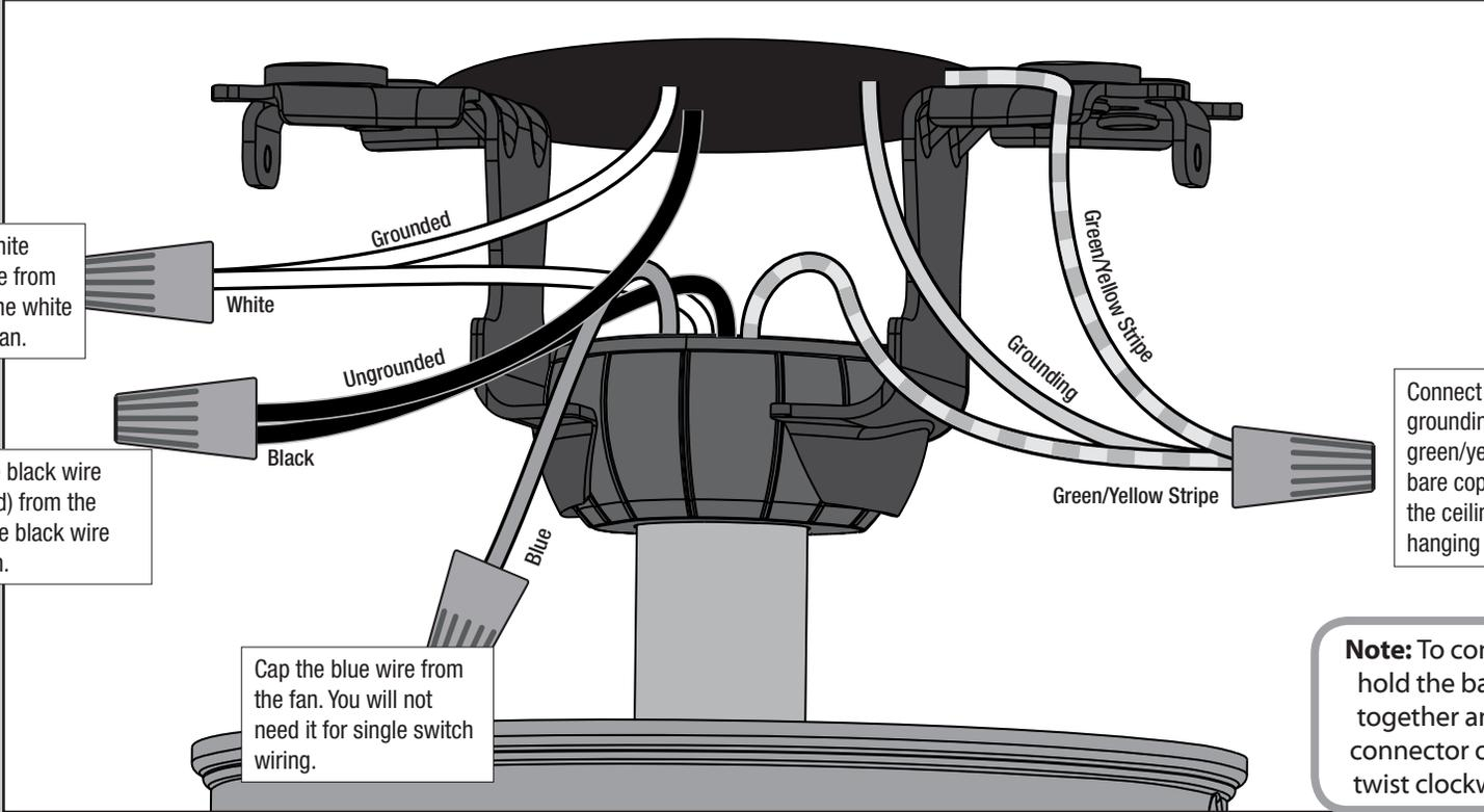
Connect the white (grounded) wire from the ceiling to the white wire from the fan.
