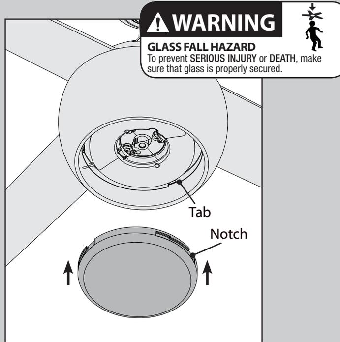
Position the notches in the outer rim of the globe so they line up with the three tabs on the inside rim of the housing. Carefully lift the globe up inside the housing as far as it will go, then rotate the globe clockwise until it is held tightly in place by the tabs.
