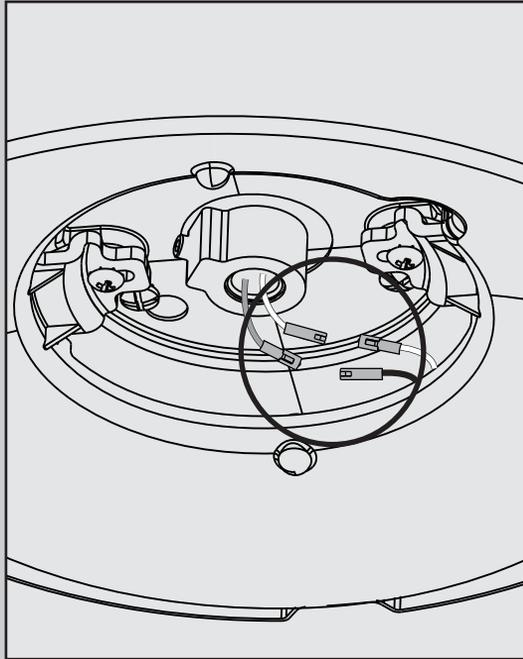
Connect the single-pin connectors from the LED assembly to the connectors from the fan. Connect the white wires together. Connect the blue and black wires together. Tuck the excess wiring above the LED assembly.
