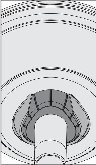
Position the canopy so that, when lifted into place, the canopy fits into the hanging bracket as shown.
