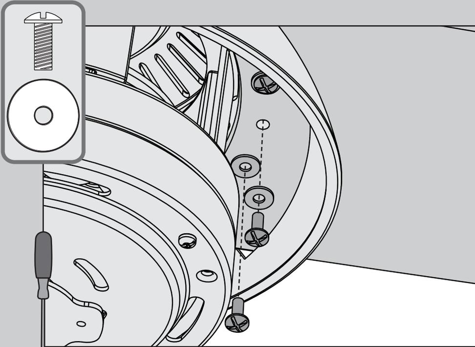
⊗ Attach the blade to the motor using the flat washers and blade assembly screws found in the ▲ hardware bag. Repeat for each blade.
