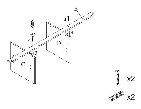
Step 3. Attach Side Panels A & B to Rail E with wood dowels and Cam locks as shown. В E point arrow on ca A 1/2 tum clockwise to fasten Attach Top F to Part A, C, D & B using wood dowels and Cam Step 4. locks as shown. Secure Rail E to Top F using Screws(Part#4) through pre-drilled holes as shown. Carefully turn cabinet over with top on the floor. point arrow on carr lock to ward adjacent hole F 13 13 3 В 13 D (4) 1/2 tum clockwise to fasten 3  $\mathsf{C}$ A
