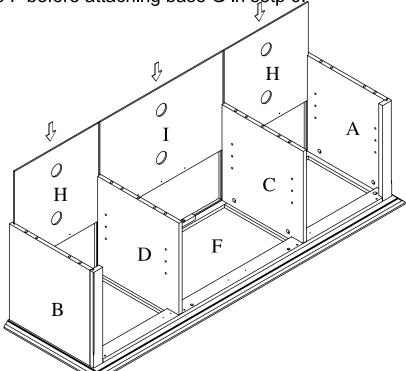
Step 6. Attach Double door magnet to the center section Rail E, and Single door magnet to both side section Rail E using Round Head Screws(Part#10) as shown. Attach Base G to cabinet using wood dowels and Allen Bolts with Spring / Flat Washer as shown. Attach legs using Hex Socket Head Bolts & Wood Dowels (as shown in instruction manual included in carton with legs).
