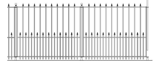
Continue adding panels, using the panel to mark the position of the next stake
