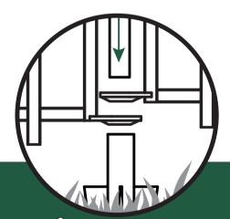
Hint: Drop post through panel rings to mark the placement for the next stake
