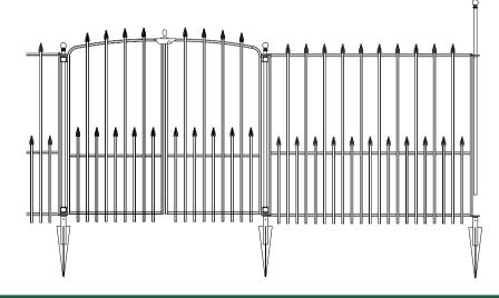
Right panel rings rest on top of left panel rings
