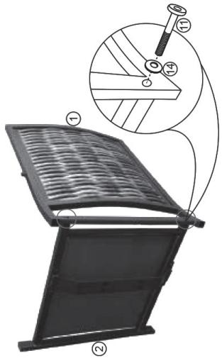
**EN:** Rotate to side. Secure hinge with washer (14) and bolt(11).
