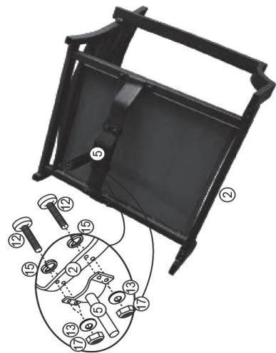
**EN:** Align Seat Post (5) with bottom of Seat (2). Insert bolt (12) in washer (15) on one end and secure with washer (13) and jam nut (17) on other end.
