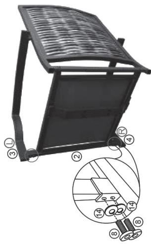
**EN:** Align Left Arm (3) with Seat (2). Secure with washer (14) and bolt (8). Rotate and repeat for Right Arm (4).
