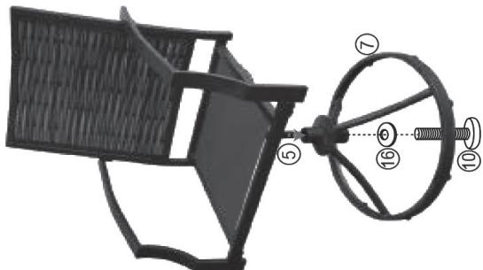
**EN:** Align assembled seat atop and insert Seat Post (5) into Base (7). Secure with washer (16) and bolt (10).
