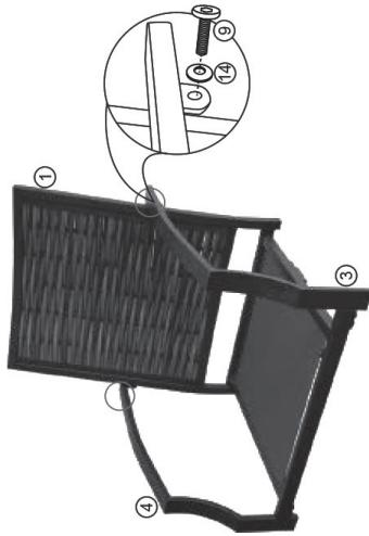
**EN:** Rotate upright. Secure Arms (3, 4) to Back (1) using washer(14) and bolt (9).
