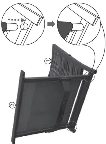
**EN:** Align Seat (2) with Back (1). Apply pressure to secure.
