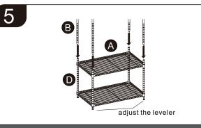
Screw the Upper Pole (B) onto the threaded ends of the Lower Poles (D). Be sure the connection is secure & tight.
