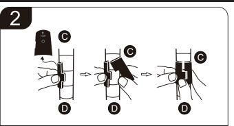
Attach 2 Spacers (C) at the pen marks on the 4 Lower Poles (D). Keep the arrows on the spacers (C) pointed upwards.
