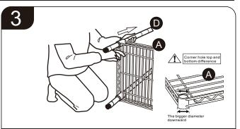
Place the Lower Poles (D) through the corner holes of 1 Shelf (A). Fit the shelf carefully and securely over the Spacers (C).
