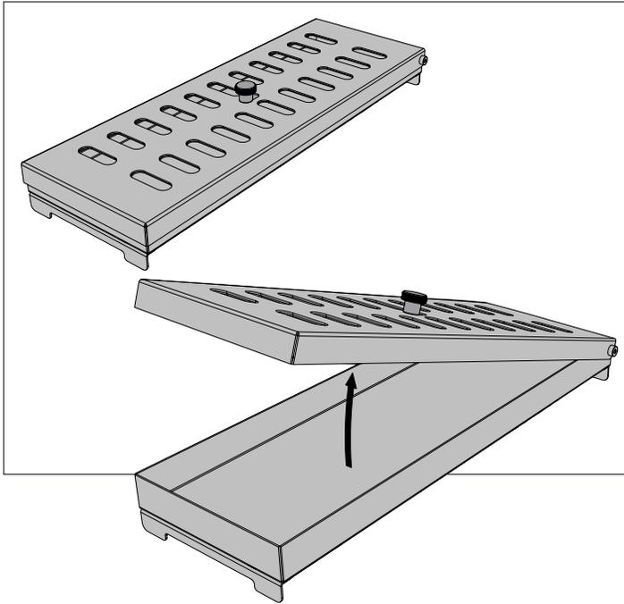
**i** Smoke vents can be adjusted by sliding the knob to control the smoke intensity.
