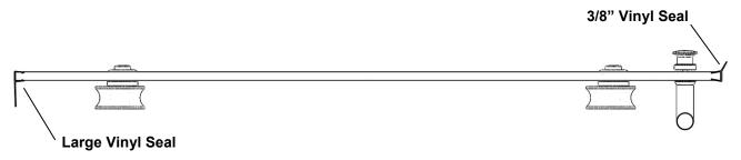
**16** The larger vinyl seal will need to be cut slightly in order for the header bar to have space to roll freely. See example below.
