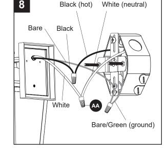
Wrap electrical tape (not included) around each individual wire connector (AA) down to the wire. Turn the spliced/taped wires upward and gently push the wires and wire connectors (AA) into the outlet box.
