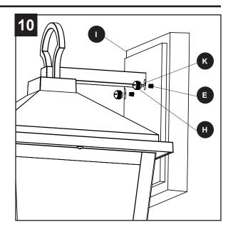
11. To prevent water, rain, or moisture from entering wall plate (I), use waterproof caulk (sold separately) to seal the perimeter.
