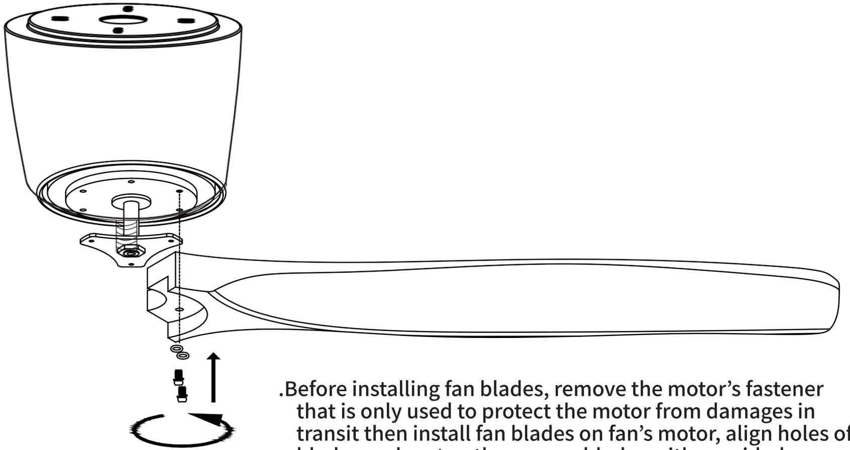
.Before installing fan blades, remove the motor's fastener that is only used to protect the motor from damages in transit then install fan blades on fan's motor, align holes of blades and motor, then screw blades with provided screws. (Figure 6)
