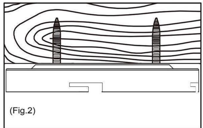
NOTE: Hanger after the installation must be able to withstand the weight of 45 kgs or more.
