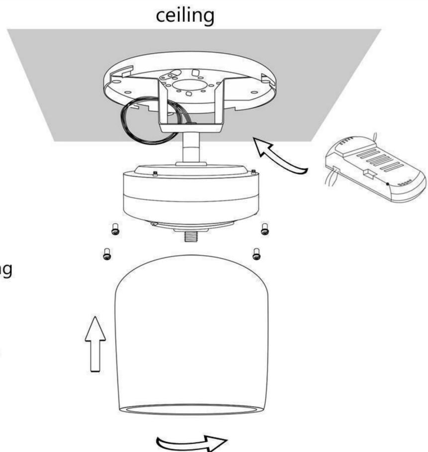
**Attention:** The lead wire must be retied tightly, otherwise it will rub against the motor and cause noise after loosening
