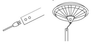
Step 4: Push the Heater Head onto the Top Tube and fix in position using the 4\*8mm screws.
