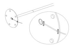
Step 6: Fix the heater on the floor. Bore three holes in the floor, fix the heater by three wedge bolts on the floor tightening the screws by spanner.
