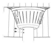
Step 5: Fix the Power Cord on the Base by using 4pcs M4 Nuts.
