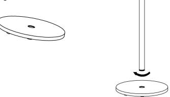
Step 2: Connect the middle tube with bottom tube by screwing them together. Connect the top tube with middle tube by screwing them together.
