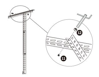
Assemble the extension rod assembly with bolts and nuts and lock with a socket wrench. Assemble 4 pairs of expansion rod assemblies in the same way. When installing, refer to the dimensions of the assembled wire grid so that the wire grid can be hung on the extension rod assembly correctly.
