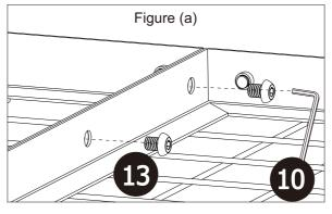
Note: To avoid the problem of misalignment of screw holes during installation, please do not tighten the screws, make sure that each one is on the right place first, then to tighten them one by one.
