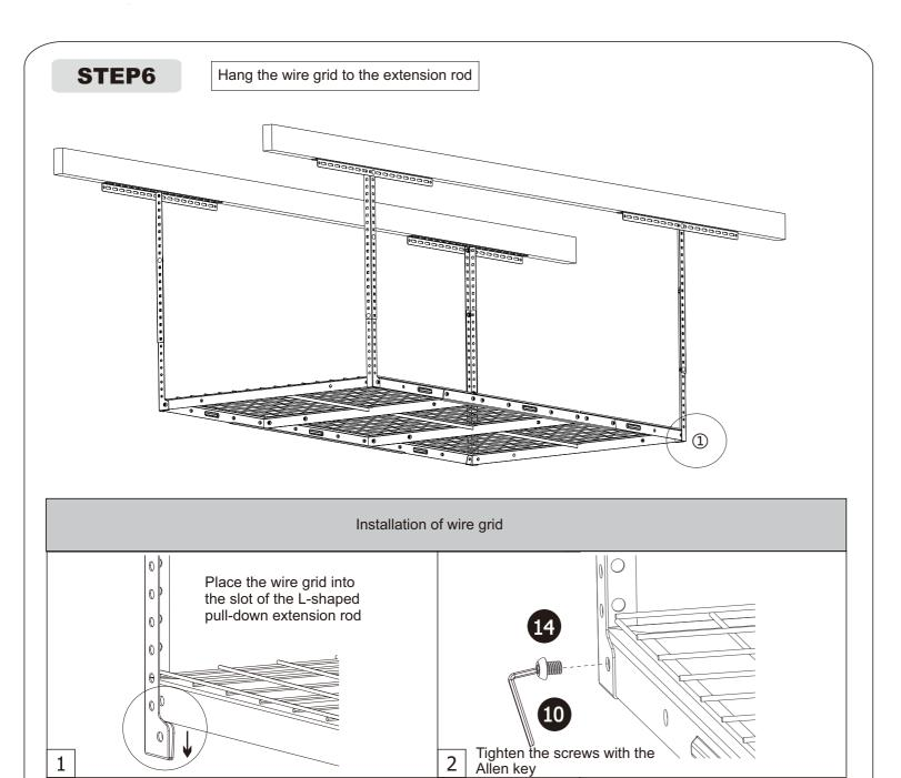
Hang the wire grid to the extension rod, connect and fix with screws as shown in the figure, and tighten with an Allen wrench.
