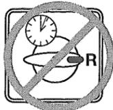
Rotation Switch controls rotation of drum only. **DO NOT USE ROTATION SWITCH REVERSE POSITION WHILE REMOVING CABLE FROM PIPE.** Use reverse direction only momentarily for relieving pressure or untangling cable from a blockage.
