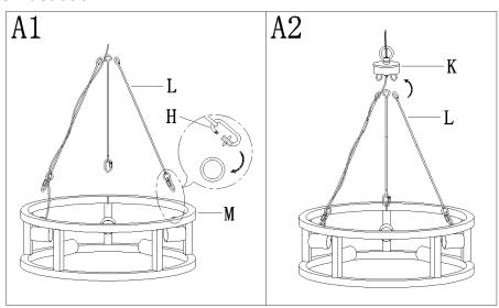
Step A1: Open quick links (H). Attach loop rods (L) to iron frame (M). Close quick links (H).
