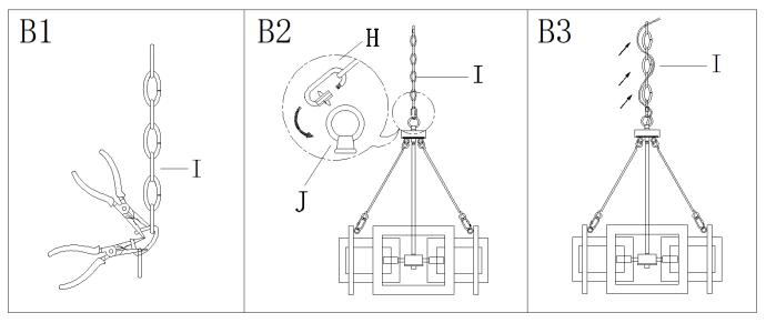
Step B1: By measuring, determine the correct number of links needed for proper hanging height. Using the chain pliers, disconnect and discard the unwanted part.
