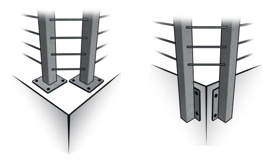
If you wrap the cable around the corner, CityPost does not recommend making more than one 90 deg or two 45 deg changes of direction with a single strand of cable as it makes achieving cable tension difficult.
