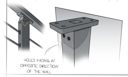
PRO-TIP: If the horizontal railing is terminating against a solid surface such as a wall or structural beam, make sure the (2) holes at the top of the post are pointed away from the
