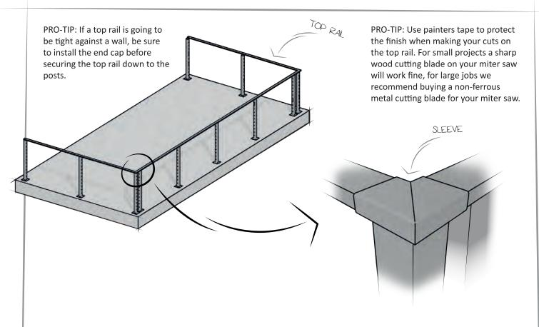
TOP RAIL COMES IN 6FT PIECES, INSTALL A STRAIGHT TOP RAIL SLEEVE OVER EACH POST, EXCEPT END POSTS. Be sure to install all bracket, sleeve and top rail screws before you begin installing cable.
