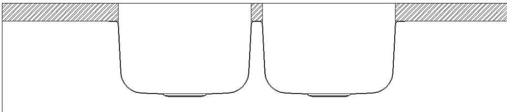
**Negative Reveal** - The counter top extends over the edge of the sink on all sides by approximately 1/4" . Use caution with this installation to be sure that accessorie such as colanders or cutting boards will fit properly .
