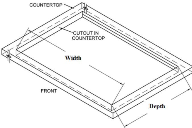
**Note:** When making the countertop, put a radius at the corners of the cutout (a radius of ¼" is typical). This will keep the countertop from cracking. Follow the countertop manufacturer's instructions regarding the minimum corner radius and reinforcement of corners.
