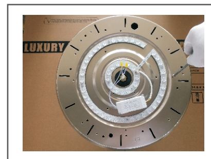
Step 4. Remove the main engine chassis screws.
