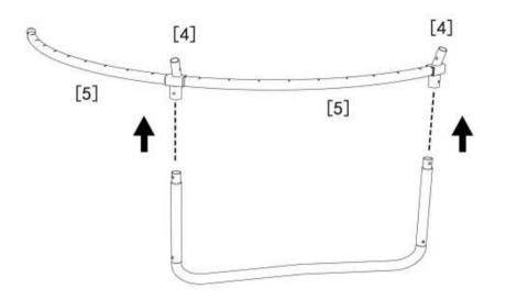
To make the hole position coincide with the metal marble position of the Leg Extension(#2) untill the metal marbles pop out and fixed.
