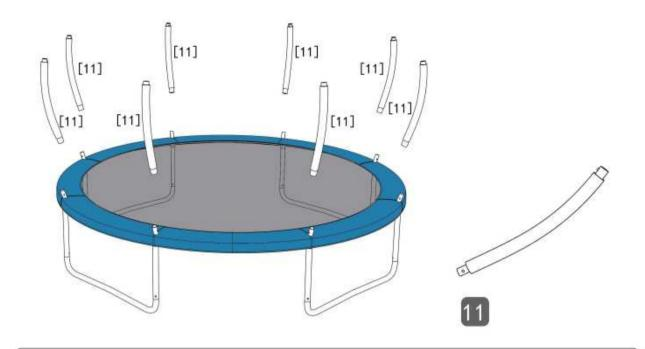
STEP 6: Mount the Bottom Safety Pole (#11) onto the Connector (#4)
