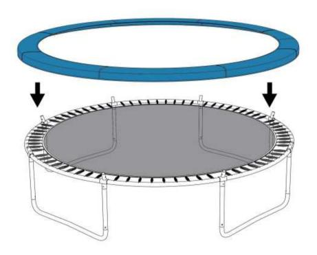
B.Tie the strap located at the under side of the frame pad to the frame.
