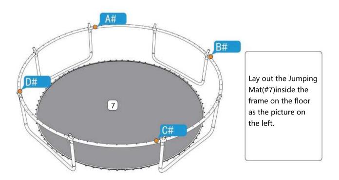
Install the Springs in the X-shape order one by one to make sure the tension is distrib-uted evenly for the Jumping Mat .Gently tap down against the spring if the hook is not completely in the hole.
