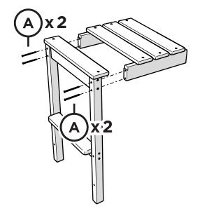
Pre-drilled holes indicate screw placement only. Fully thread screws into material for full engagement
