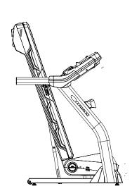
7. Make sure that the locking mechanism is engaged. Carefully pull back on the walking deck and make sure that it does not move. When you do this, keep clear of movement path in case the treadmill lock is not properly engaged.
