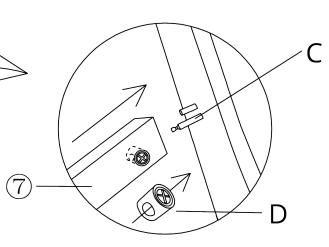
Firstly, fix two screw nuts (D) to the bottom slats (7), then fix (7) to the chair legs.
