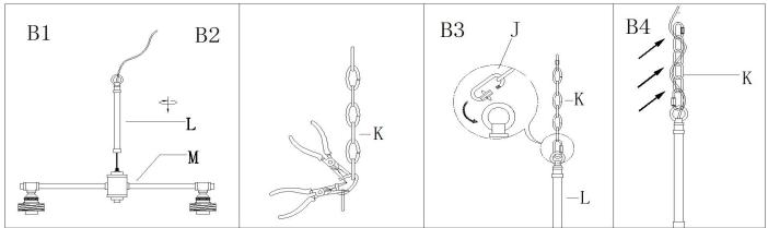
Step B1: Thread the tube (L)onto the fixture body (M) till tight .
