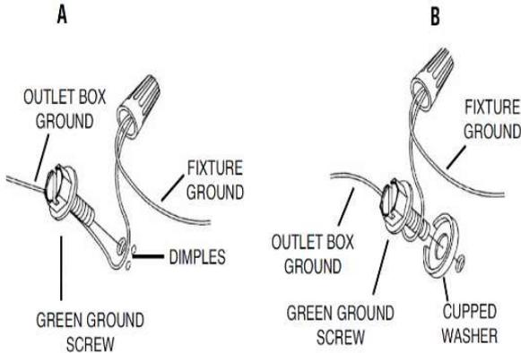
**Connect wires according to below chart**
