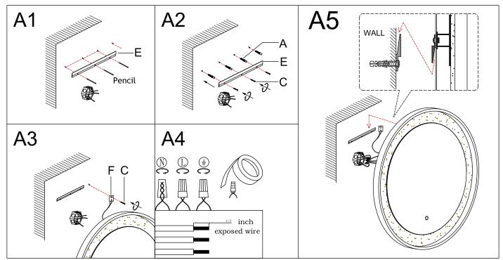
Step A1» 1) By measuring, mark spots on the wall and above the outlet box with a pencil, and draw a total of 4 spots.
