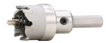
The 1-1/8-Inch Carbide Hole Cutter is ideal for cutting 3/4-Inch conduit and pipe. It features a split-point pilot drill bit to reduce walking. An integrated flange helps prevent drilling beyond the sheet metal.
