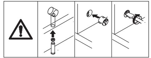
Connect board 6 to board 4, add cam lock(B) into and turn clockwise to tighten as shown. Insert bottom board 5 along grooves as shown.
