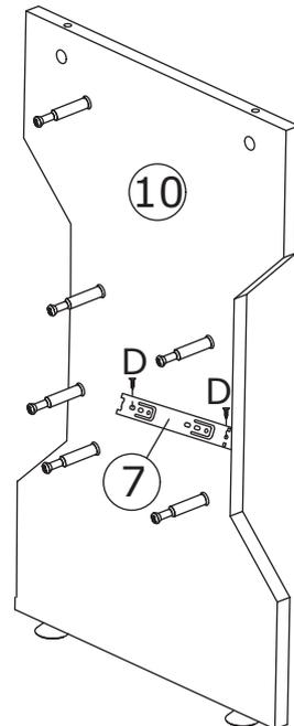
Fix rail part 7 to board 9 and 10 with screw(D) as shown.
