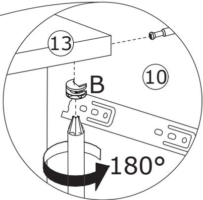
Attach board 13 to board 10, add cam lock(B) into board 13 and turn clockwise to tighten as shown.
