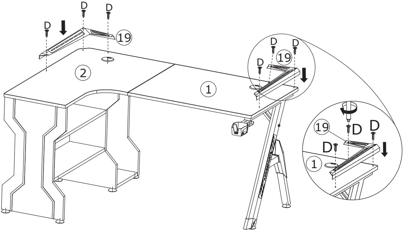
Fix part 19 to board 1 and 2 with screw(D) as shown.
