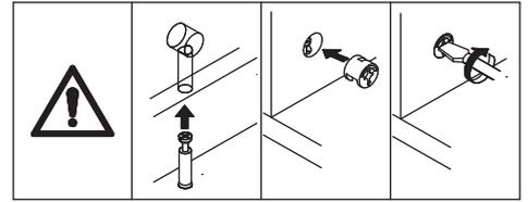
Attach board 9 to board 13 and 16, add cam lock(B) into board 13,16 and turn clockwise to tighten as shown.
