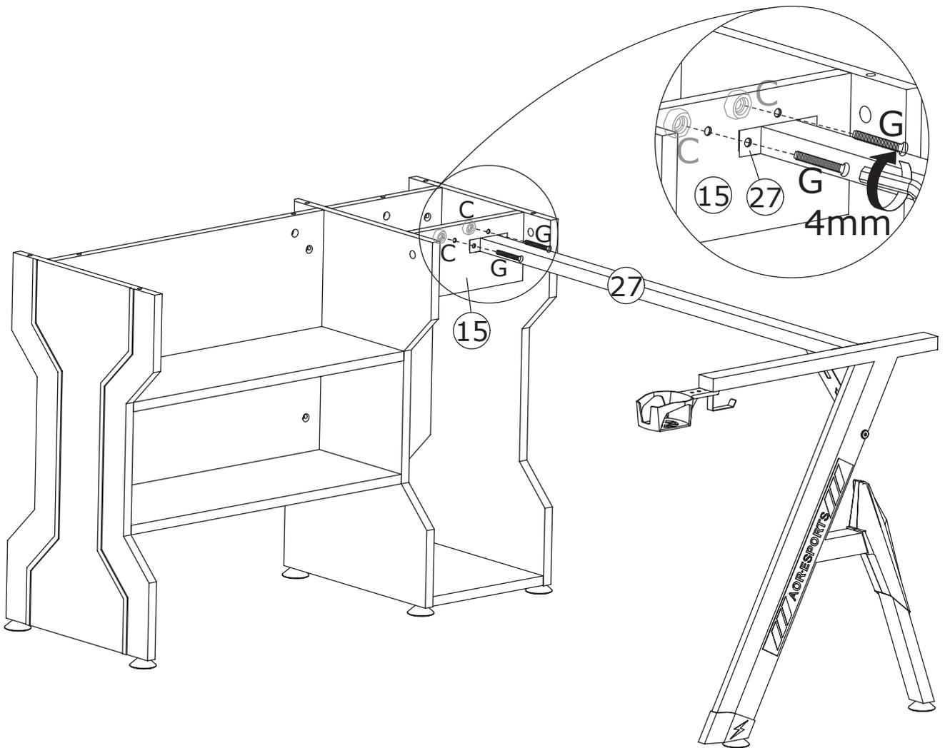
Fix part 27 to board 15 with screw(G) and nut(C) as shown.
