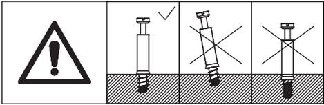
Screw eccentric rod(A) into board 11 as shown.
