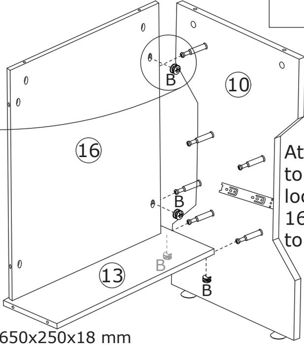
Attach board 13 and 16 to board 10, add cam lock(B) into board 13, 16 and turn clockwise to tighten as shown.
