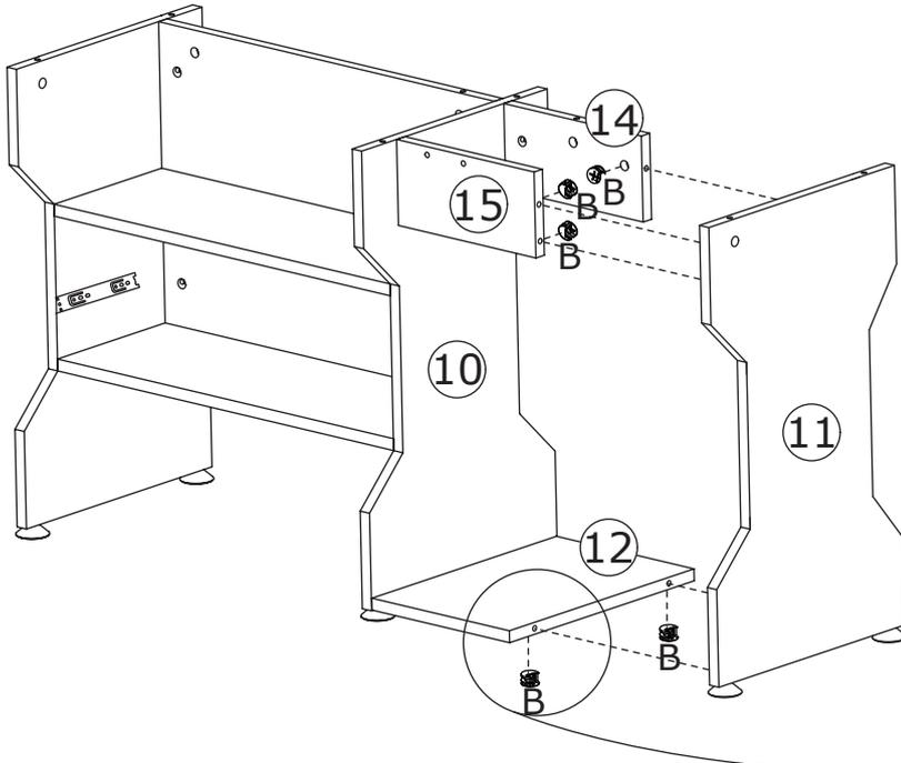
Attach board 11 to board 12, 14 and 15, add cam lock(B) into board 12,14,15 and turn clockwise to tighten as shown.
