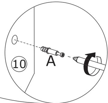
Screw eccentric rod(A) into board 10 as shown.
