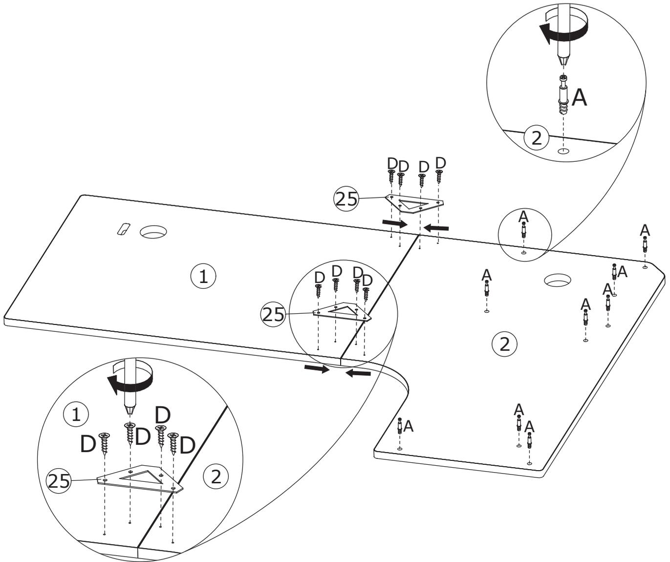
Screw eccentric rod(A) into board 2 as shown.
