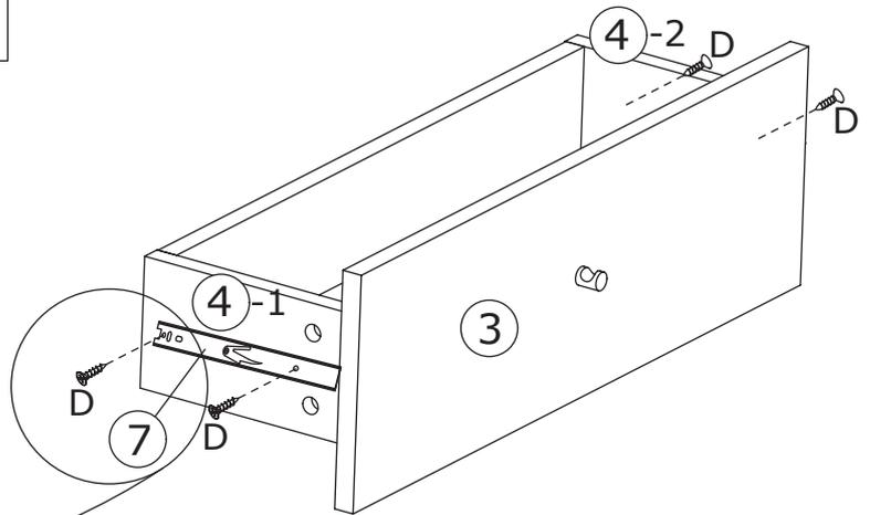
Fix runner part 7 to board 4 with screw(D) as shown.
