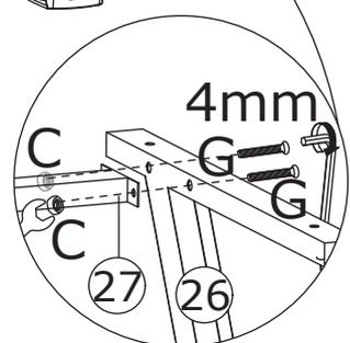
Fix part 28 to part 26 with screw(E) and nut(C) as shown. Fix part 27 to part 26 with screw(G) and nut(C) as shown.
