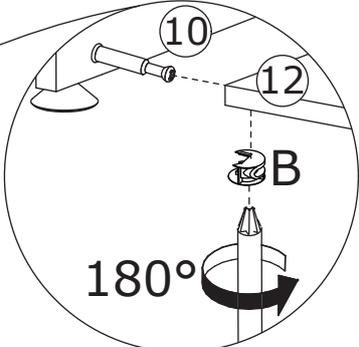
Attach board 12, 14 and 15 to board 10, add cam lock(B) into board 12,14,15 and turn clockwise to tighten as shown.
