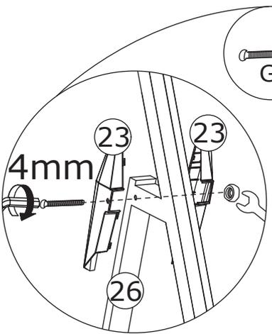
Fix part 23 to part 26 with screw(G) and nut(C) as shown. Fix part 20 and 21 to part 26 with screw(F) as shown.
