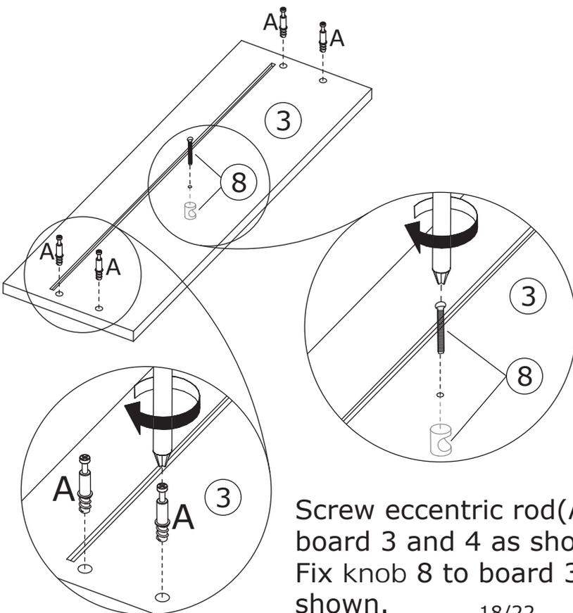
Screw eccentric rod(A) into board 3 and 4 as shown. Fix knob 8 to board 3 as shown.
