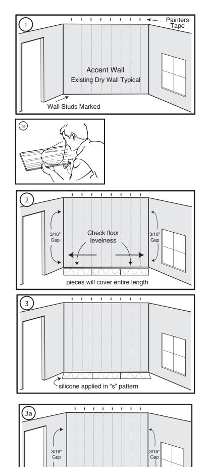
Drive a brad nail into each plank at each wall stud through the shallow area of the extended groove (see inset diagram). Take care that the brad nail heads are not raised, but also don't force them all the way through the groove. This will allow easy connection of the next row of planks. You must also place drywall screws every 16" into the wall studs or sill plate along the bottom edge of the first row of planks where they will be covered by the wall base. (Figure 4)
