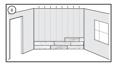
For the last row of the installation, use painters tape to mark the stud location for brad nailing. Cut all planks in the last row to the required width to complete the installation. Complete the installation as you have the earlier rows. (Figure 8a)
