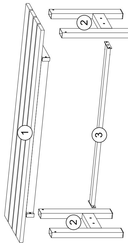
**EN:** Do not tighten the screws during installation, tighten them after all parts have been installed.
