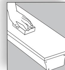
**ALL SURFACES:** Holes, depressions, and indentations should be filled with a wood filler and raised areas sanded smooth.
