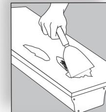
**OLD SURFACES:** When applying face veneer over old finishes, first clean thoroughly with denatured alcohol and allow to dry. Surface should be sanded and free of dust, oil, grease, wax, paint and other foreign matter. Surface should be sealed with a light coat of wood sealer for best adhesion. Allow sealer to dry completely.
