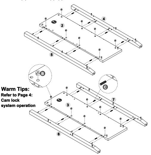
Warm Tips: Make sure the 4 large pre-drilled hole are on the upside (4)&(5) holes should be in the same side.
