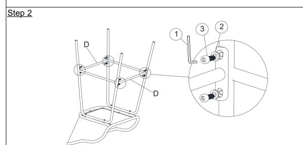
Attach the Support Bar (D) to Left Leg (B) and Right Leg (C) using Bolts (③) and Washers (②) with Allen Wrench (①) as shown above.
