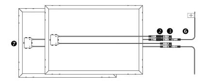
Connect the positive bare wire end 6 to the "+" PV input of the charge controller 1.
