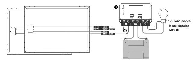
Remove the panel covering. In good sunlight, the charge controller's • "BAT %" should increase to 100%. When the controller is set to "LOAD ON," the system will provide power through the load control output or through the USB port.
