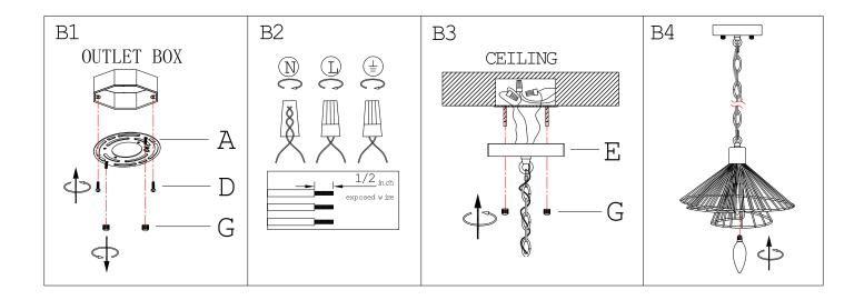
Step B1 » 1) Attach mounting plate (A) to the outlet box with mounting screws (D).
