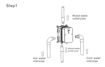
As shown in the figure, the inlet and outlet pipes are pre-buried,pay attention to the correct direction of installing the pre-buried box, and make sure that the mark TOP on the top of the installation box is facing upward.
