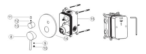
Please fix the ®Main body to the wall then remove the plastic protective cover and install @Panel ® Water divider, ® Screw,® Water divider cup in the order. Finally you could install & Handle, 9 Screw, Mandle cup.
