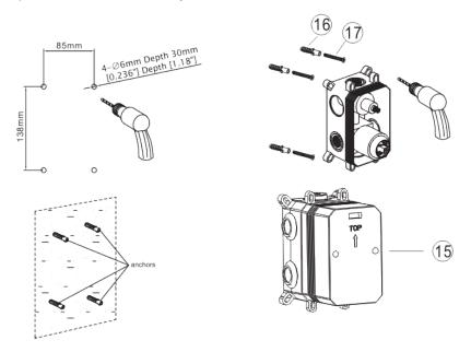
Please note that the level meter should be parallel, otherwise the panel cannot be installed Pay attention to the length and width of the screw position before marking
