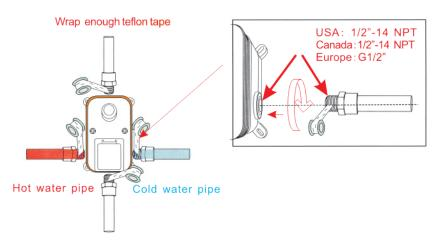
Install the hot and cold water inlet pipes, Shower head and hand shower holder pipes. Turn on the water source to test whether the left and right inlet pipes are tightly connected without leakage. After the test, adjust the flow switch to be on to test whether the mixed outlet pipe. The connection is tight and there is no leakage.
