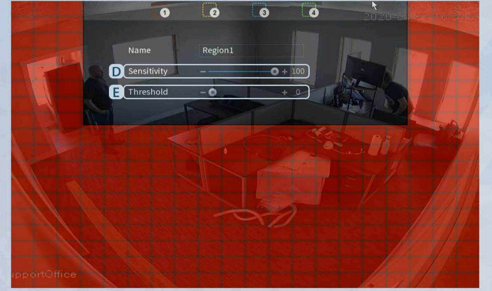
Some cameras are equipped with SMD (Smart Motion Detection). SMD allows the camera to filter notifications to events caused by a human or vehicle. To enable SMD you will select 'Al' from the main menu and then choose 'Parameters' from the left hand column. Then select 'SMD' below the parameters. Enable SMD and then choose if you want it to apply to Human, Vehicle, or Both. Finally select 'Apply' to save your configuration. Masking
