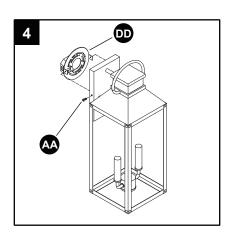
CAUTION: To avoid any waterproofing problems, please make sure the light fixture fits the mounting surface perfectly installation and use waterproof glue around the canopy for better sealing after installation.
