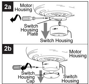
Punch center cap out of switch housing or switch housing cap with a screwdriver (not included).
