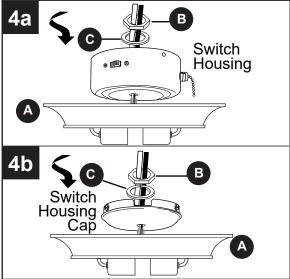
5a. Remove wire connectors from WHITE and BLUE (or BLACK) wires labeled FOR LIGHT in switch housing. Connect WHITE wire from light kit fitter (A) to WHITE wire from fan. Connect BLACK wire from light kit fitter (A) to BLUE (or BLACK) wire from fan. Use wire connectors that were previously removed to make the connections.
