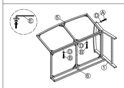
STEP 7: Connect The Part from Step (6) & Back Bench (5), tighten Allen Bolt (A), (B), Flat Washer(D) with Allen Key (E).
