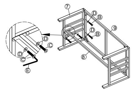
STEP 13: Connect Support Bar (8) & The Part from Step (12), tighten Allen Bolt (C),Flat Washer(D) with Allen Key (E).
