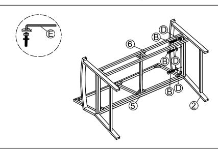
STEP 8: Connect The Part from Step (7) and Left Frame (2), tighten Allen Bolt (B), Flat Washer (D) with Allen Key (E).
