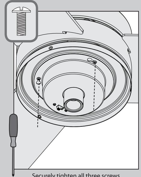
⊗ Securely tighten all three screws.
