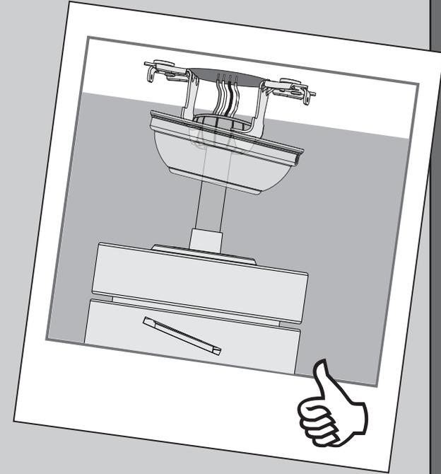
**Note:** To connect the wires, hold the bare metal leads together and place a wire connector over them, then twist clockwise until tight.
