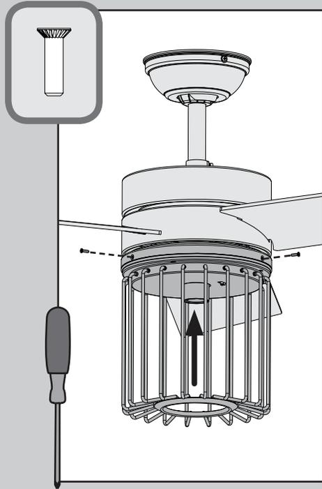
⊗ Lift the cage and attach it to the upper switch housing using the three screws. Be sure to align the hole in the cage assembly with the reverse switch. Tighten all three screws securely.
