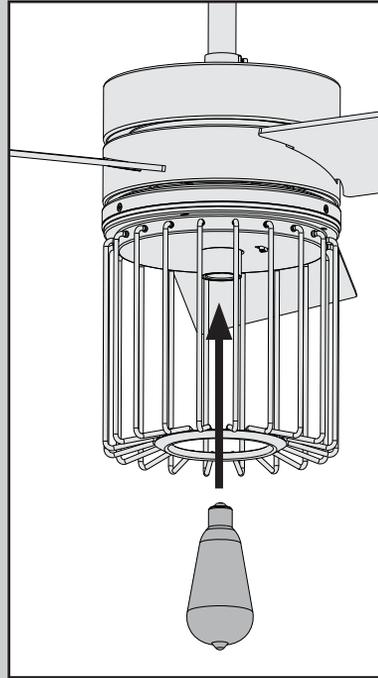
Install a bulb into the socket. When necessary, replace with a bulb of the same type and wattage.
