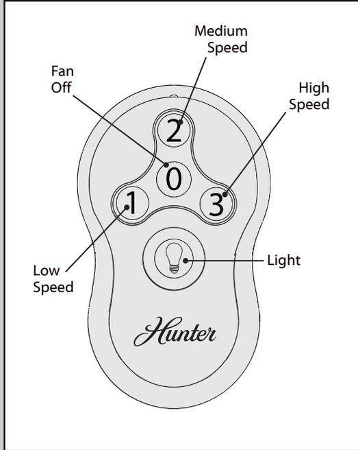
To turn on fan, press a fan speed button. Speeds range from off (0) to high (3). Quickly press the Light button to turn the lights off and on.
