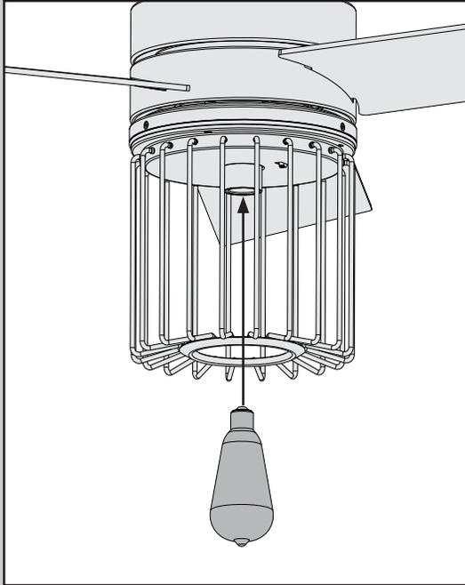
**Changing the bulb** - Unscrew the bulb and replace with a bulb of same type and wattage.
