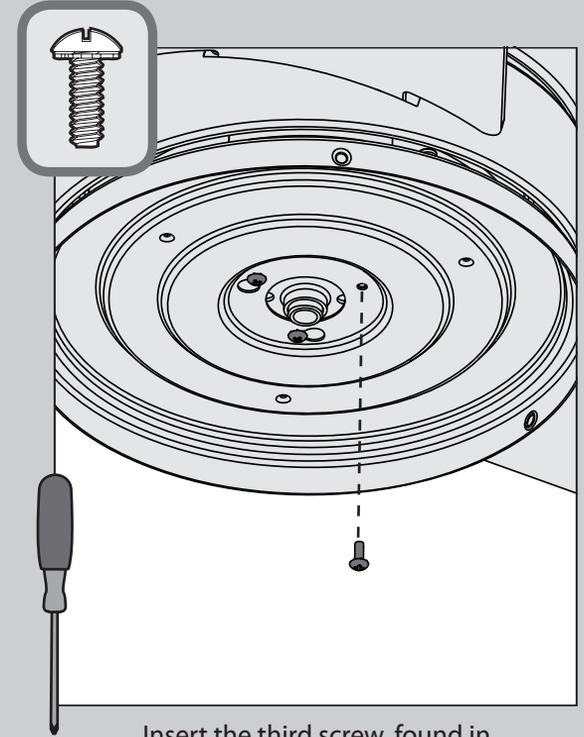
⊗ Insert the third screw, found in the ≡ hardware bag, into place and then tighten all three screws.
