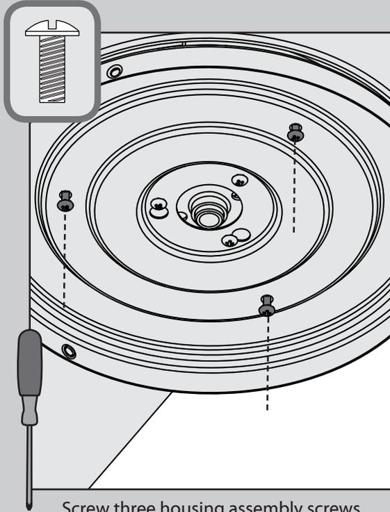
⊗ Screw three housing assembly screws from the ≡ hardware bag halfway into the upper switch housing.
