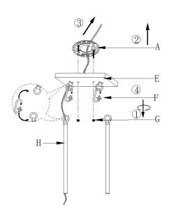
6. Pass the wires from outlet box through the mounting plate (A) Attach the mounting plate(A) to outlet box with the mounting screws (D)
