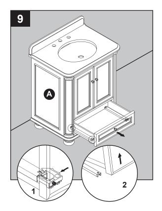
10. To re-install drawer into vanity (A). Please fully extend metal glide tracks, gently lower and slide drawer box into rear glide catch, then, lower drawer box down to completely rest on extended glides, push plastic levers to lock the drawer box in place.
