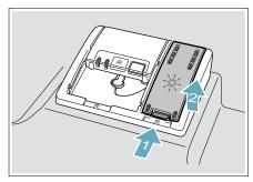
Add liquid rinse aid to the dispenser 32 until it is full. Do not overfill. Avoid spilling into air vent hole.
