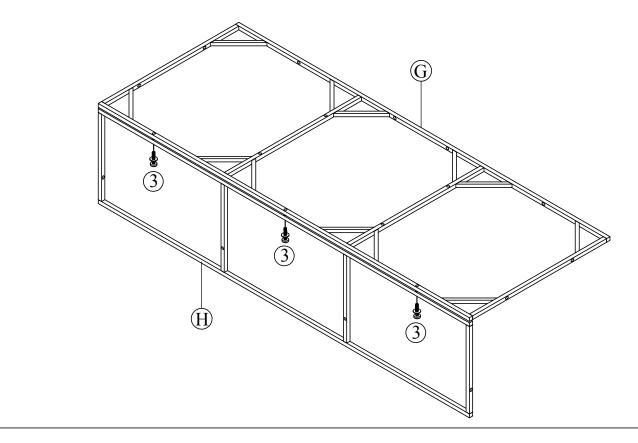
Connect Part from STEP 7 & Hip Support Frame (I) with Bolt (3) & Washer (5)
