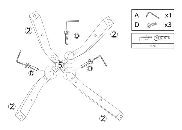
First install the footrest ③ and tighten its screws to 80%. Then tighten all screws on footrest ③ to 100%. Finally tighten all screws on connecting frame ⑤ to 100%.
