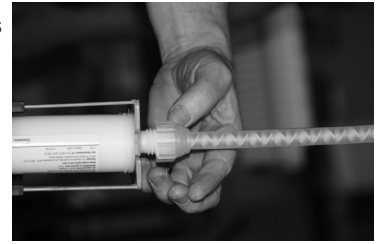
FIGURE 14: ATTACH STATIC MIXING TIP
