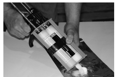
FIGURE 13: LEVELING THE PLUNGERS
