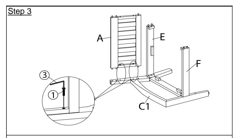
Insert dowels on Backrest Panel(A) into mountings on Left Arm Panel(C1). Attach Left Arm Panel(C1) to Backrest Panel(A) using Bolts(1) with Allen Key(3). Do not fully tighten the Bolts.
