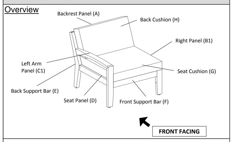
This Left Chair has multiple parts and may require up to 30 minutes to assemble. To give you an overview of the Left Chair parts, the above picture is to help you put the various parts into perspective. Please read through the instructions below to familiarise yourself with the parts and steps before assembly.
