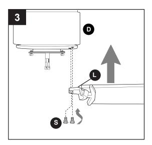
Locate motor screws/washers (S) that were previously removed (Step 5, page 7).
