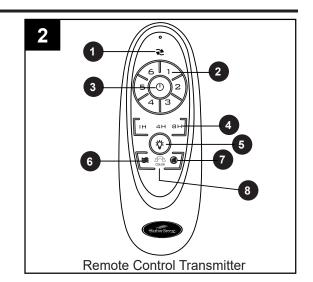
Tap button quickly to turn lights off or on. Hold button down to increase or decrease light. If you press  $2^{\circ}$  button in excess of 7 seconds, it becomes a dimmer. The light varies cyclically in 8 seconds. The 🖞 button also has an auto resume function which: (1) keeps the light at the same brightness as the last time it was turned off, and (2) resumes at the same speed as the last time it was turned off.
