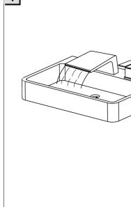
Installation finished; Turn on faucet, check all connections for leakage; Re-tighten them if necessary.
