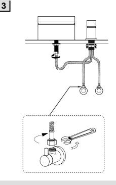
Connect the other side of red and blue water supply lines to the correct angle valves and use wrench to tighten them; Connect the other side of mixer water supply line to the spout and hand tight it(Don't use wrench in case of thread damage!)
